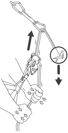
Place the rope in the braking groove A, accompany it towards the device with both hands and lower the climber.
