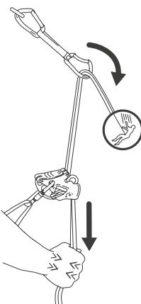
Hold the free end of the rope firmly in one hand and pull it downwards. Don't hold the device in your hands!
