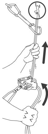
With one hand, bend the free end of the rope, with the other pull and feed the climber's rope through the device.
