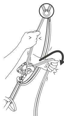
Take up the slack as instructed under the point 6.2. and use your own weight to tension the ropes and the device.
