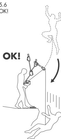
When ascending a multi-pitch route, the rope must pass through a directional anchorage on the belay point.
