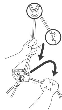
With one hand pull and feed the free end of the rope through the device, with the other pull the climber's rope towards it.
