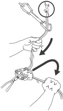
With one hand pull and feed the free end of the rope, with the other pull the climber's rope towards the device.
