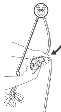
Belay yourself to the belay station using a sling, connect the karabiner to the belay loop and insert the rope in the device.
