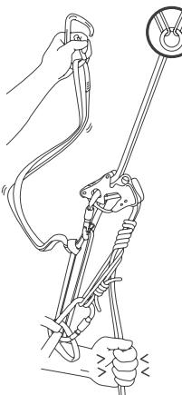
With one hand hold firmly the free end of the rope, then release the sling and disconnect the karabiner from the belay station.
