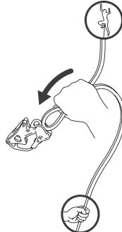
Insert the loop of the rope in the slot B, referring to symbols 2-6-8 on the device. With single rope, use the slot opposite the karabiner gate.
