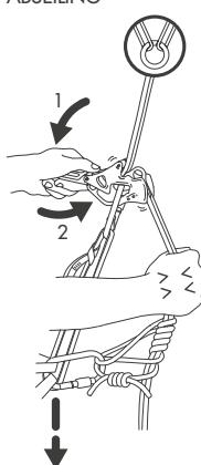
To practice to abseiling in a self-locking way, make a Prusik knot on the rope below the device.
