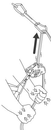
Grasp the rope firmly with both hands and move them alternately downwards to lower the climber to the ground.
