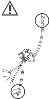
Alpine Up is positioned correctly but the rope is inserted in a wrong way: **stop immediately the ascent!**
