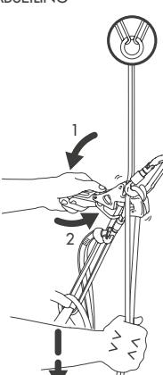
Open the lever H (1), press on it and rotate the device upwards (2). Pull the free end of the rope towards the device, so to abseil.
