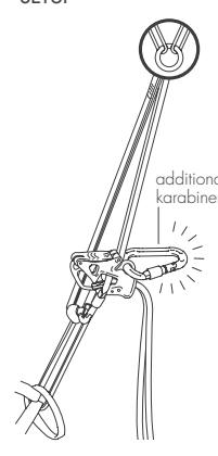
Install the device as instructed under point 8.1-8.2, then insert an additional locking karabiner in the hole I.
