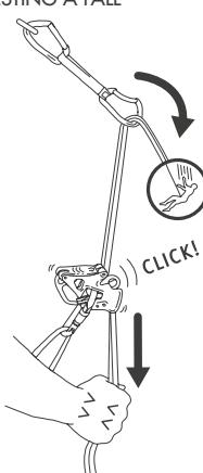
Hold the free end of the rope firmly in one hand and pull it downwards.
