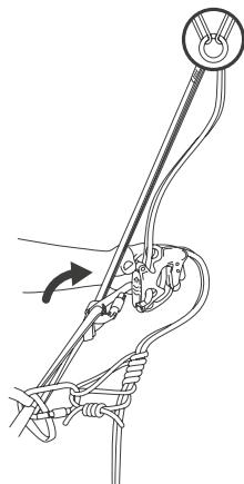
Belay yourself to the belay station, install the device as in 12.1÷12.4 and tie a Prusik knot on the rope below the device.
