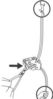
Insert the karabiner in the hole F with the rope inside. Close the karabiner gate!
