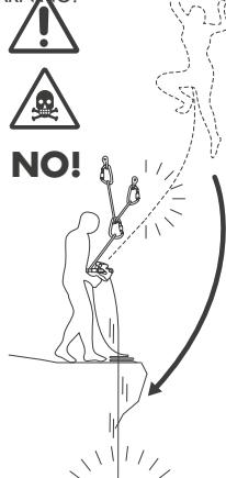
Always pass the leader rope through a directional anchorage, on the belay station.
