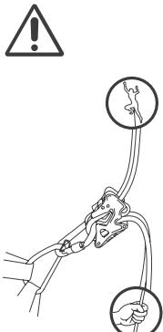
Alpine Up is positioned incorrectly and the rope is inserted in a wrong way: **stop immediately the ascent!**
