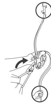
Insert the karabiner at right angles to the lever H in the hole G with the rope inside. Close the karabiner gate!
