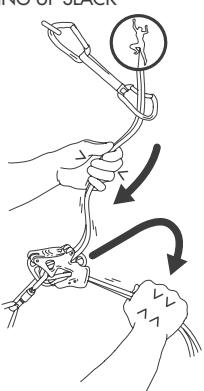
With one hand pull the free end of the rope through the device; with the other pull the climber's rope towards the device.
