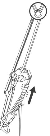
Tension the knot with both hands so that you can be suspended on the rope.
