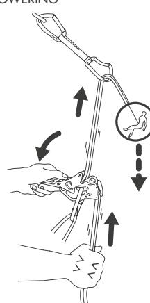
Open the lever H and push it downwards, with the other hand feed the free end of the rope through the device.
