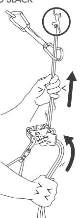
With one hand, bend the free end of the rope and feed it through the device; with the other pull the climber's rope.
