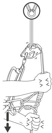
Control the Prusik knot with one hand on the rope; with the other hand control the rate of descent.
