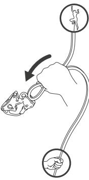
Insert the loop of the rope in the slot B, referring to symbols 2-7-8 on the device. Close the karabiner gate!
