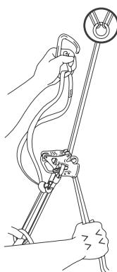
Hold the free end of the rope in one hand, with the other release the sling karabiner and hook it to the gear loop in the harness.
