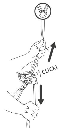
Before starting climbing, take up slack [Fig. 5.2] and activate the device in lock mode.
