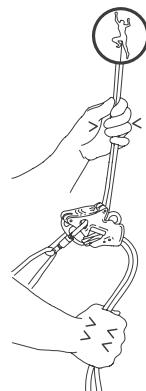
The system is OK. From now on always hold firmly the free end of the rope in your hand!
