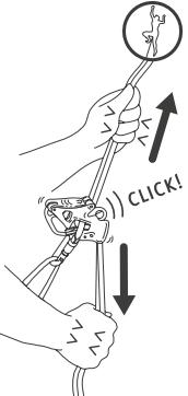
Check the device works correctly before use, verifying that it locks the rope with a typical "CLICK" sound.
