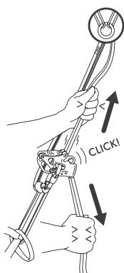
Install the Alpine Up in the sling and activate it in lock mode as instructed under the point 5.2.
